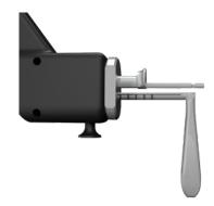
Confirm Guide Pin position and remove the Guide Pin Sleeve. Attach the Lag Screw Drill to power and insert into the Lag Screw Drill Sleeve over the 3.2mm Guide Pin. Drill to the depth measured for the Lag Screw. The calibrations are read off the back of the drill sleeve. Confirm the Lag Screw Drill tip position under fluoroscopy.
